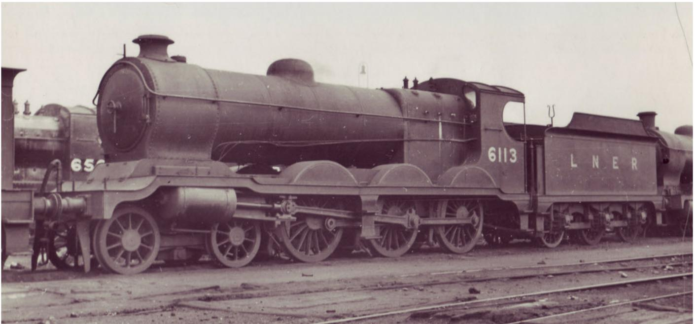
Robinson Class 8G, B9/2 '6113' in LNER days. This engine has been superheated (evidence the rivets around the smoke box wrapper, the Gresley 'snifter' and the whistle on the fire box) but the wheel on the smoke box door is still fitted. The date is after 1925. Note the pseudo - GCR chimney for the LNER loading gauge. Apart from a raised pitch of 4" during superheating this engine looks almost as it was when built in 1906 apart from some obvious untidyness and wear.
