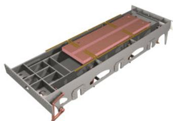
The final version of the frame shown here with the current collecting PCB fitted. There is plenty of space for both lead weights and a DCC chip.
