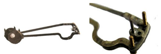
The prototype - with through hole drilled to 2.4 mm
