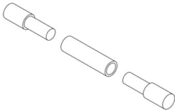
The modified centre axle. The valve gear is trapped between the brass tube and the ends and is therefore fixed. Some care is needed getting the dimensions correct but once done the wheels can be fitted over the ends and quartered normally.
