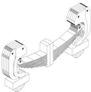
In the later version the two single holes have been replaced by a single fixing point for a 14 BA or 16 BA countersunk bolt through the frames and the top layer is partly half etched away so that it fits as an overlap on the bottom of the frames.
