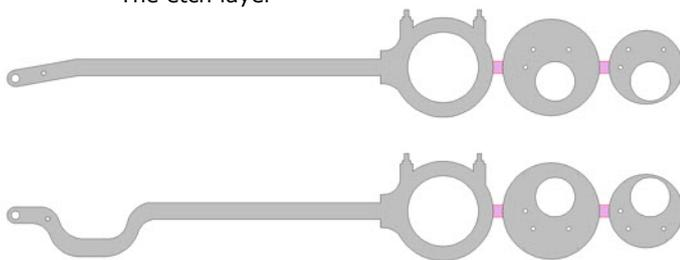
The initial plan was to do all of this in 0.35 N/S etched parts and on the face of it, it should have worked. The outline for the etch is shown, the pink bits are the usual tags.
