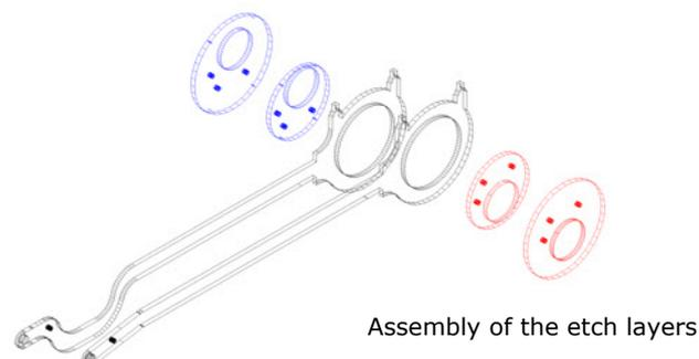
Assembly of the etch layers
