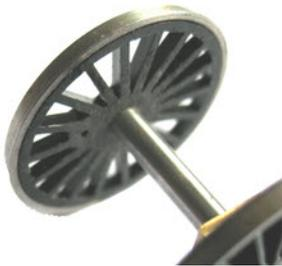
The modified Gibson wheel - fix some masking tape around the spokes area and use a graver or very sharp knife to gently remove the surplus. Use very fine wet and dry to finish, brush clean and then fit the crank pins and wheels as usual.
